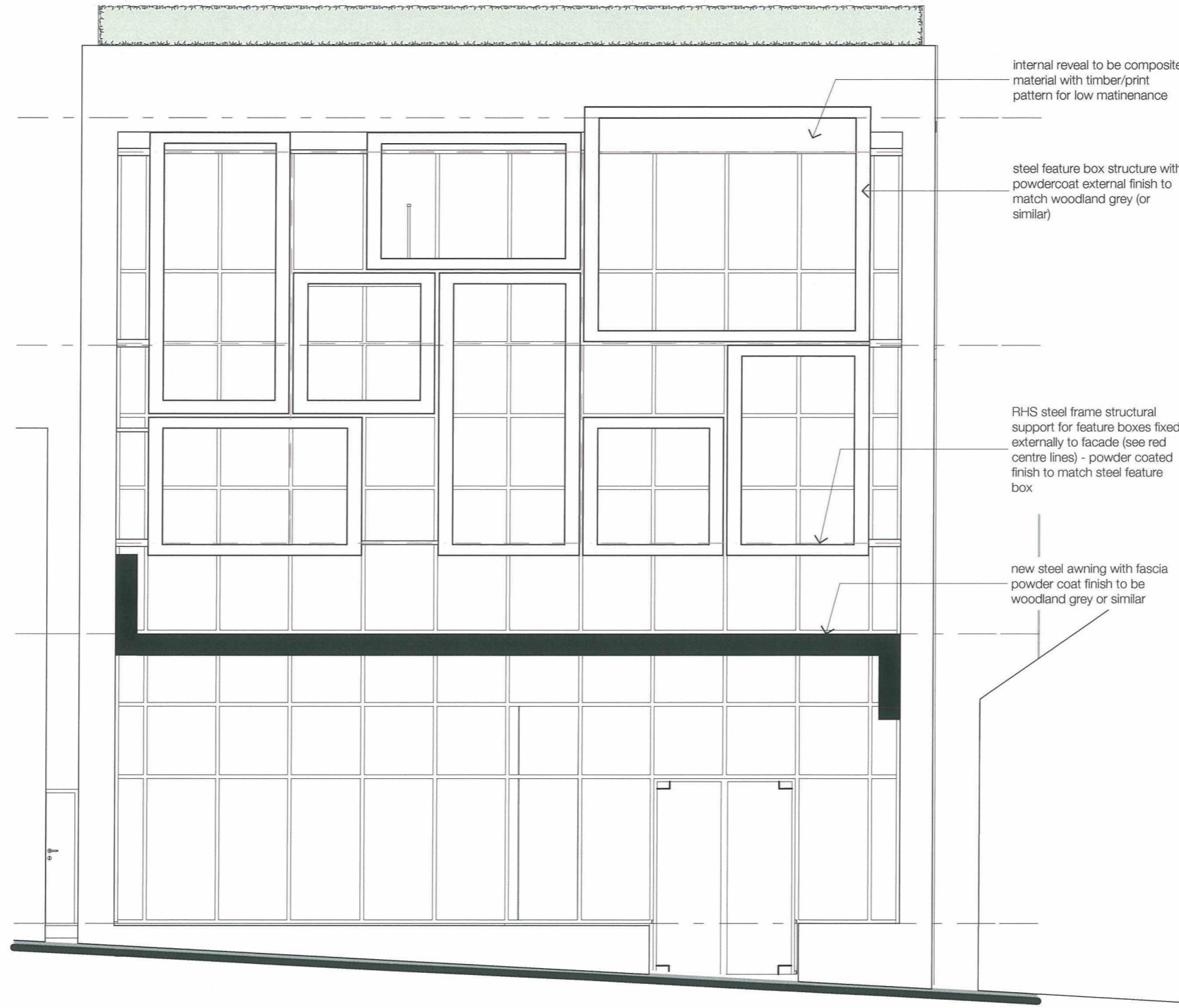
3 | box frame elevation detail 1:50
