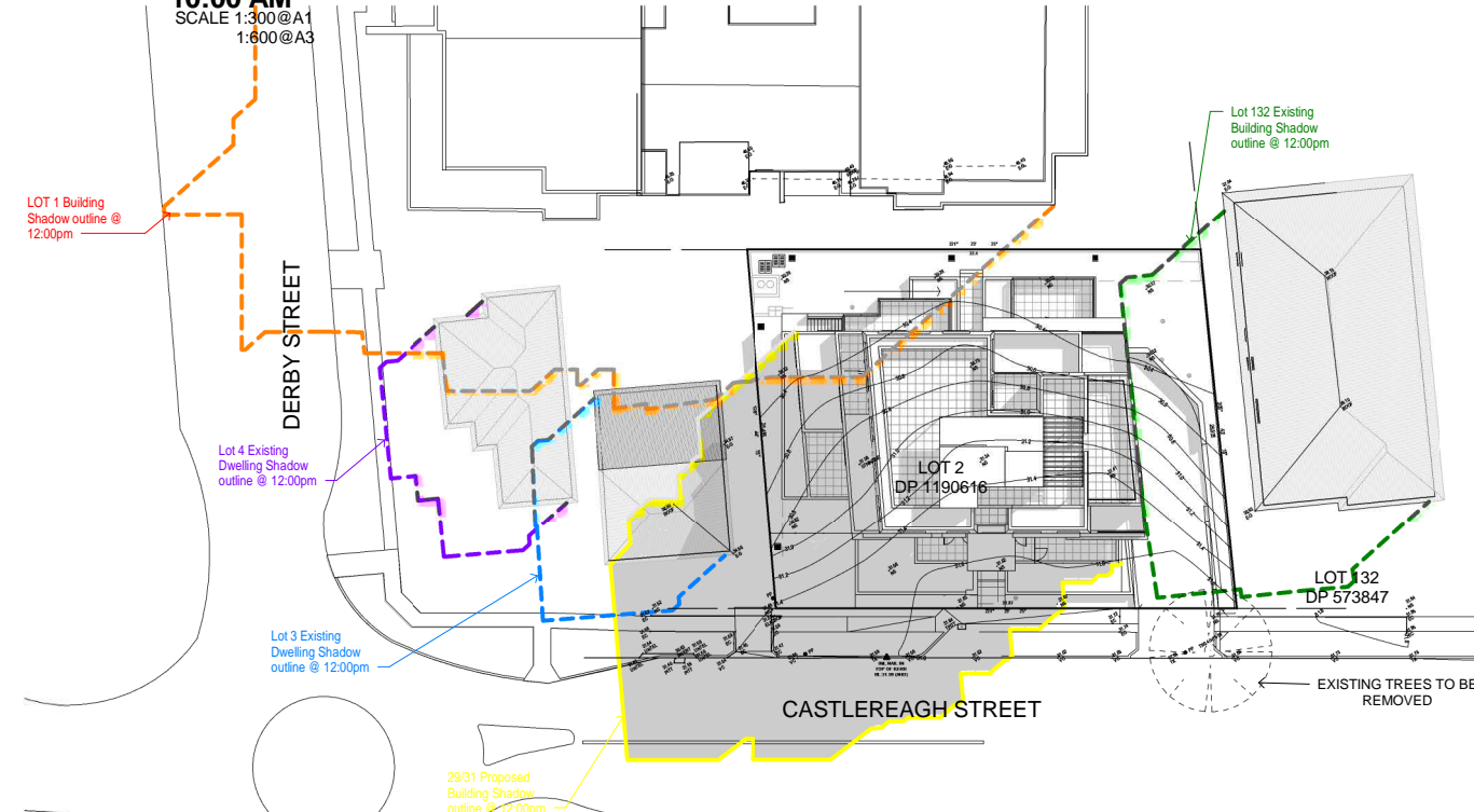
SHADOW DIAGRAMS WINTER SOLSTICE JUNE 21 12:00 PM SCALE 1:300@A1 1:600@A3
