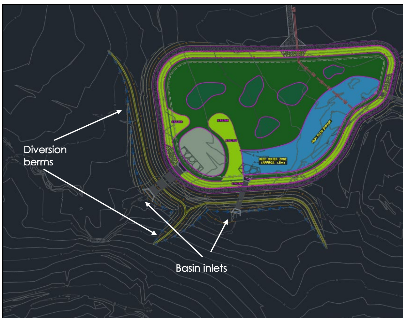
Figure 4. Basin C inlet and berm configuration
