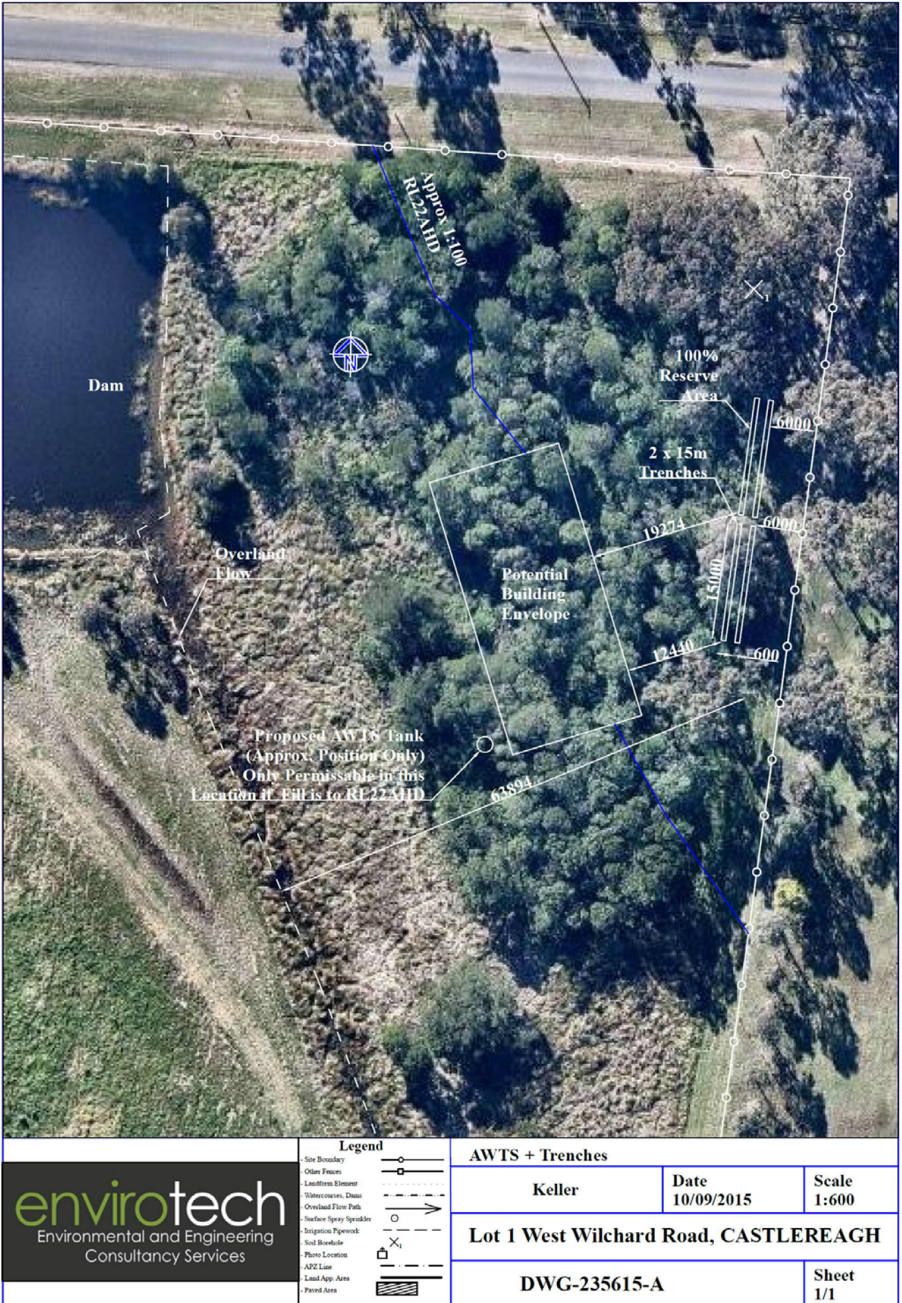
Figure 3: On site wastewater management system design.
