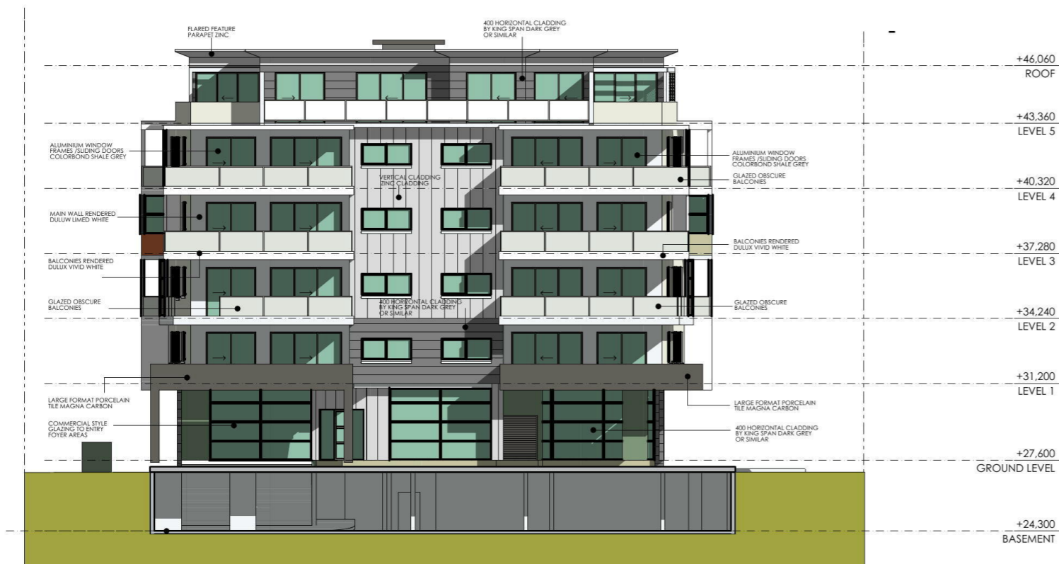
3 NORTH ELEVATION BLOCK B 1:250
