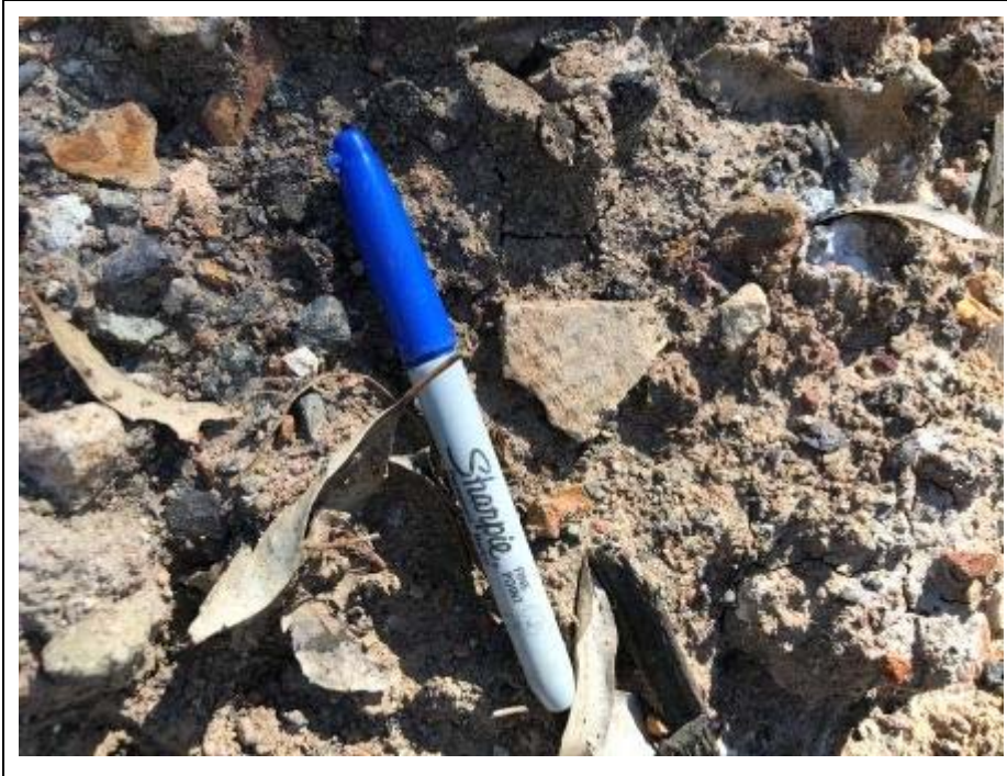
Image 6.10.2 View of example of fragment of FCS on surface of stockpile on site
