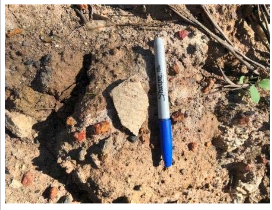
Image 6.10.3 View of example of fragment of FCS on surface of stockpile on site
