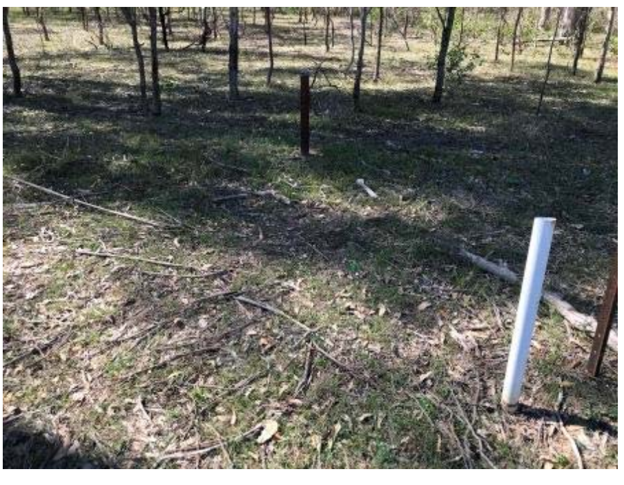
Image 6.2.5 View of two groundwater monitoring wells (PVC and metal) in south western corner of the site
