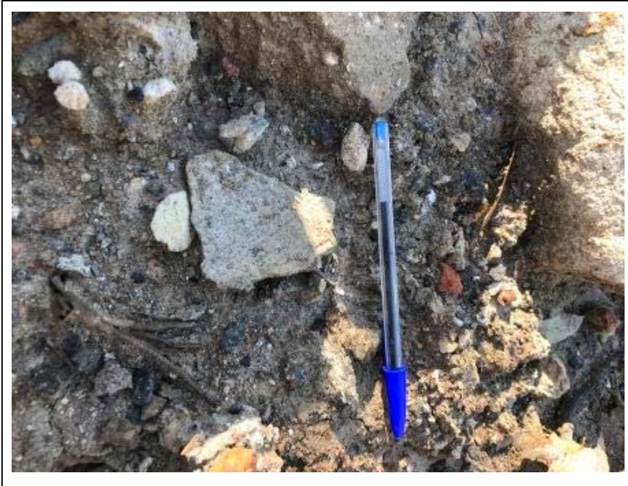
Image 6.10.4 View of example of fragment of FCS on surface of stockpile on site
