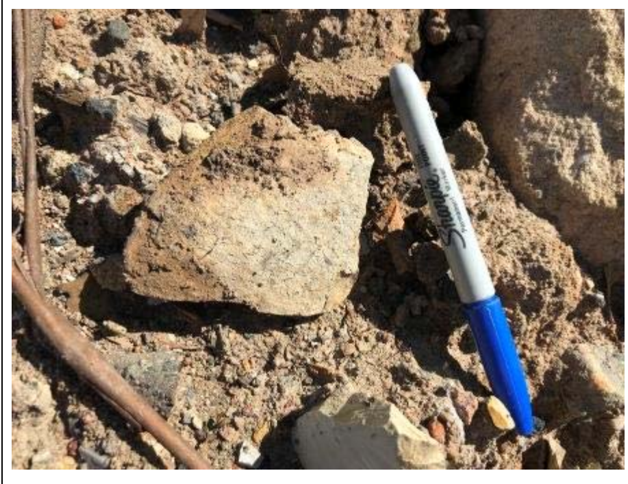
Image 6.10.1 View of example of fragment of FCS on surface of stockpile on site
