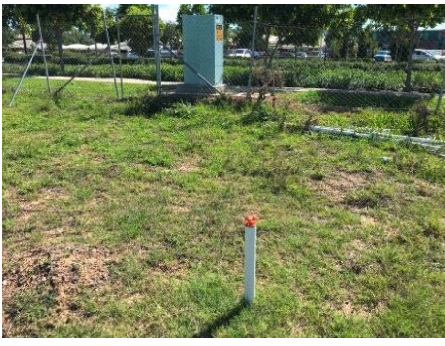
Image 6.2.5 View of two groundwater monitoring wells (PVC and metal) in south western corner of the site
