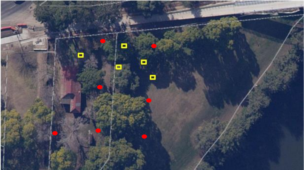
Figure 1 Location of test trenches (yellow) and contamination testing pits (red) associated with the location of the Punt House
