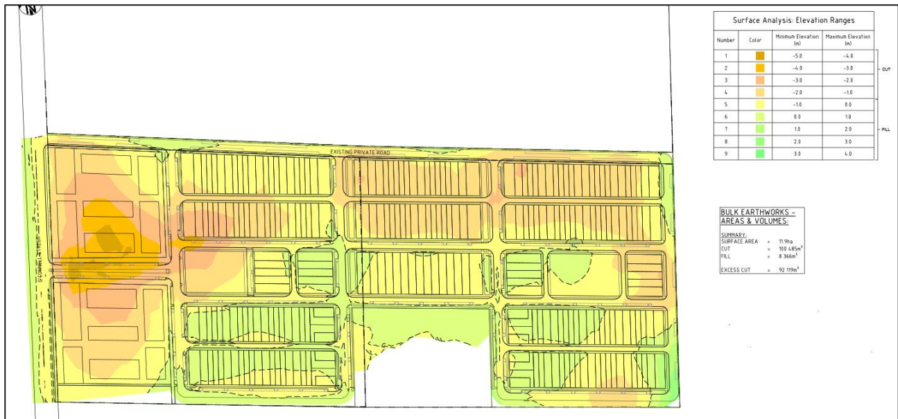
Figure 12 – Indicative Cut and Fill Quantities
