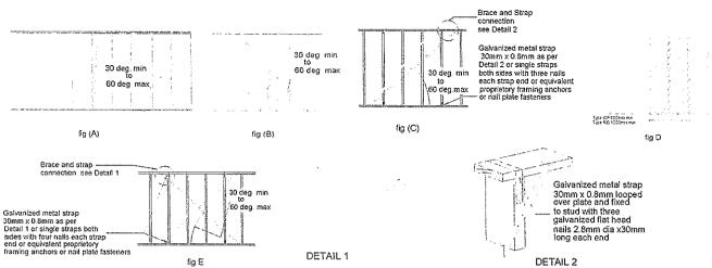
Diagrams as shown and explanation of the various types of bracings are not intended to specify bracing requirements for any timber frame construction. All bracing requirements for a particular design in timber framing must be determined in accordance with Section 8 of AS1684.2 or AS1684.4 as applicable.
