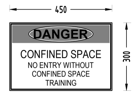
9 DETAIL CONFINED SPACE SIGN NOT TO SCALE
