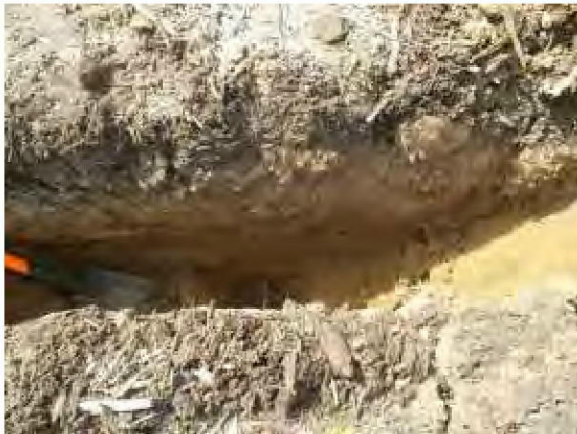
Photo 10. Test pit showing fill with natural soil observed at depth.
