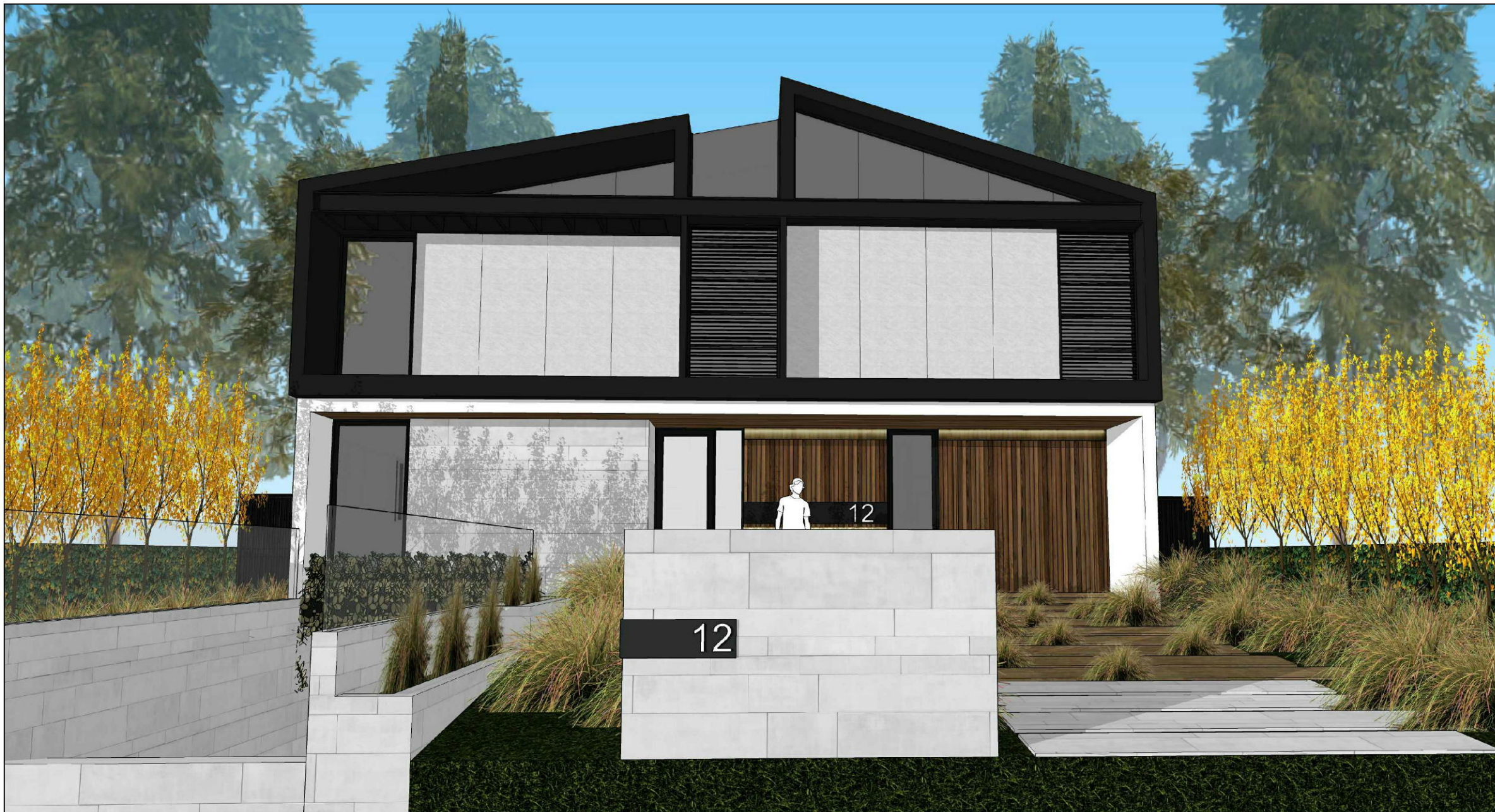
GARAGE DOOR/ CEDAR CLADDING COLOUR : STAINED
