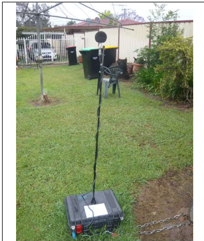
Figure 5.2 – Acoustic Monitor in Position at Site
