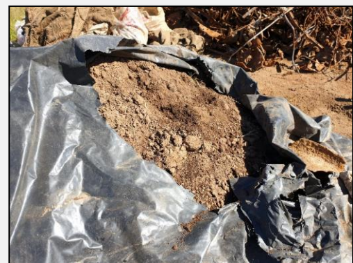
Photo 18: 19 March 2020: General soil material encountered within stockpile of residual asbestos impacted soils.
