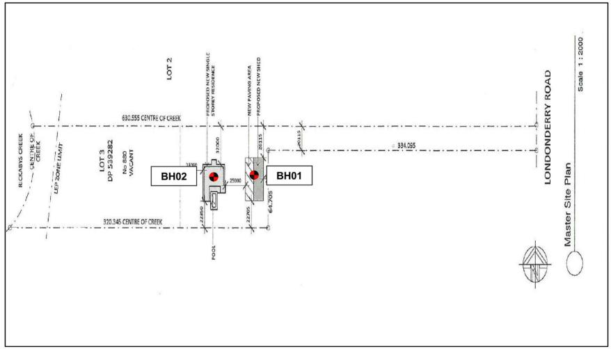
Note: Boreholes not to scale. Borehole/test location approximate. DCP undertaken in all borehole locations.
