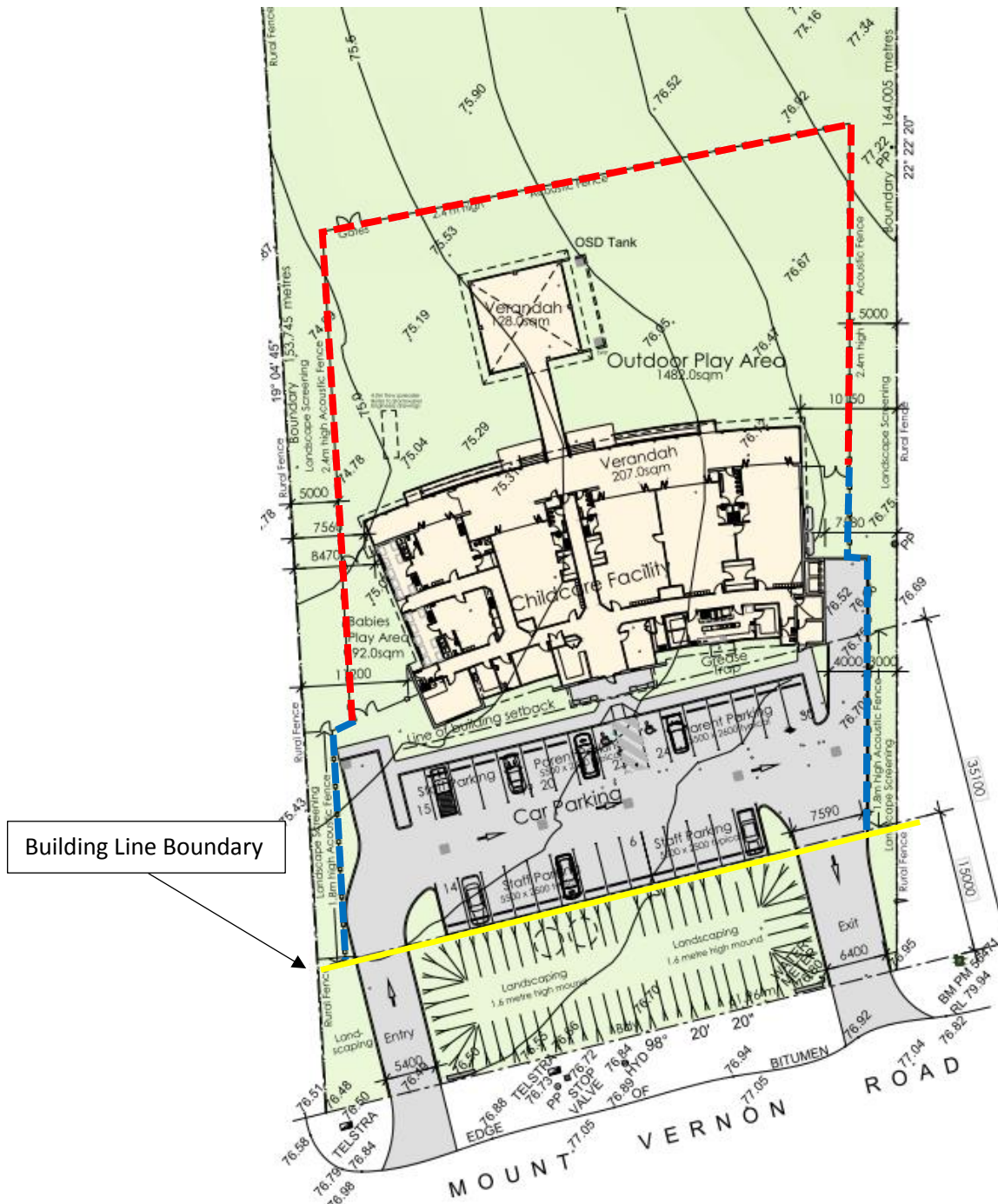
Figure 8-1: Boundary Fence Mark-up
