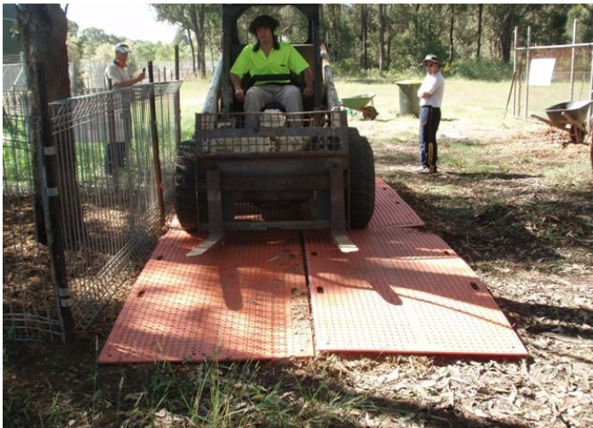
Photo 9: The load-sharing surfaces should be designed to take the load that will travel over it.
