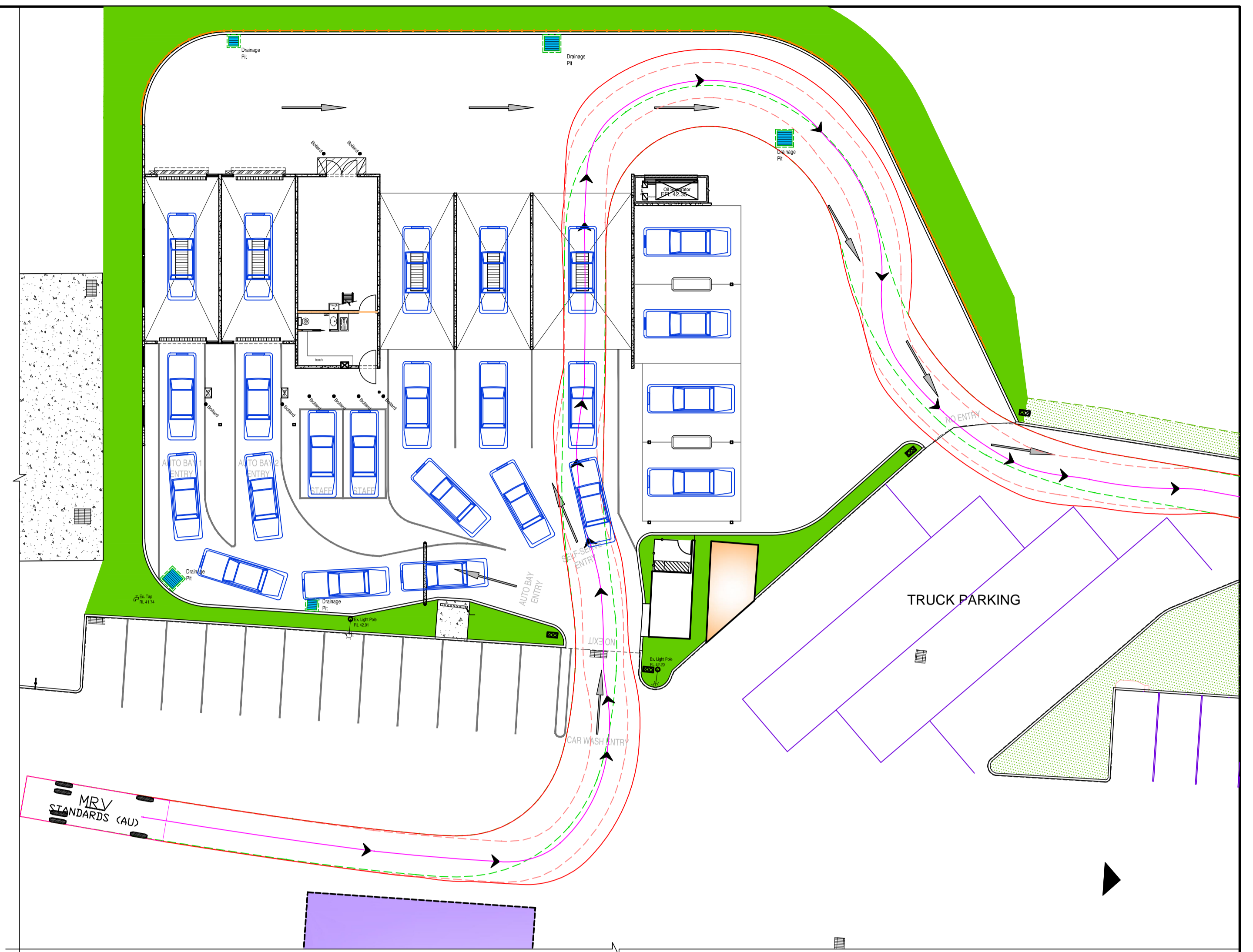
MEDIUM RIGID VEHICLE SWEEP PATH & GENERAL PARKING LAYOUT
