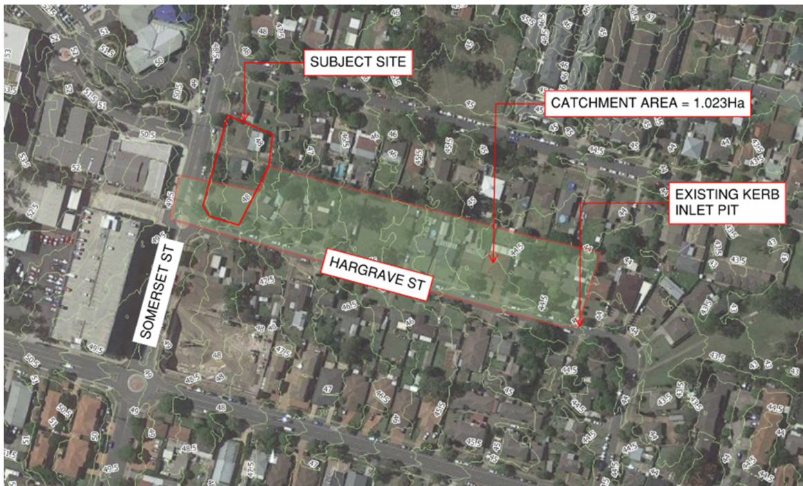
Figure 3: Catchment of the existing kerb inlet at Hargrave St.
