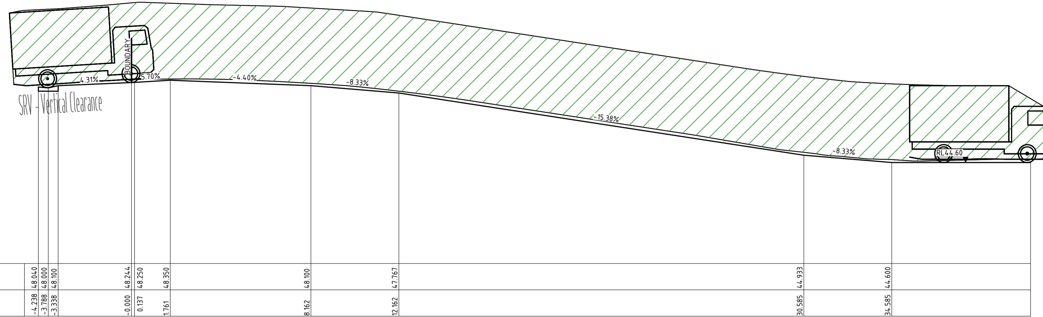
DRIVEWAY LONGITUDINAL SECTION 1 DESIGN VEHICLE 6.4m SRV
