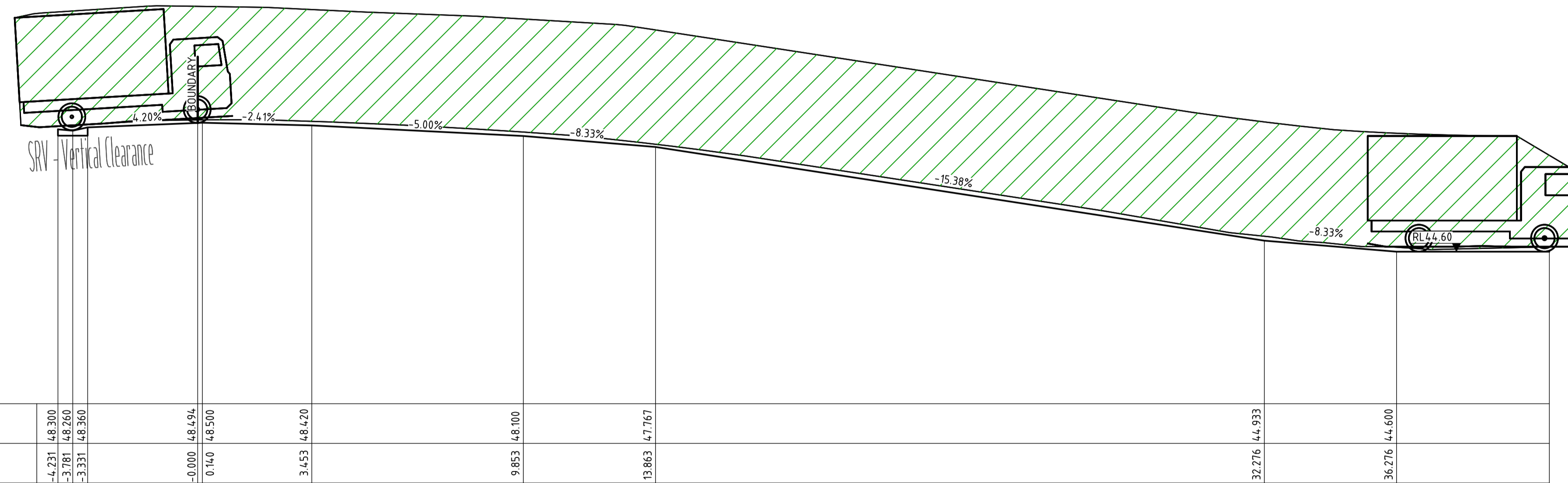
DRIVEWAY LONGITUDINAL SECTION 2 DESIGN VEHICLE 6.4m SRV
