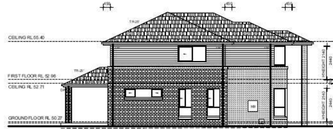
1:100 SIDE ELEVATION (NORTH)
