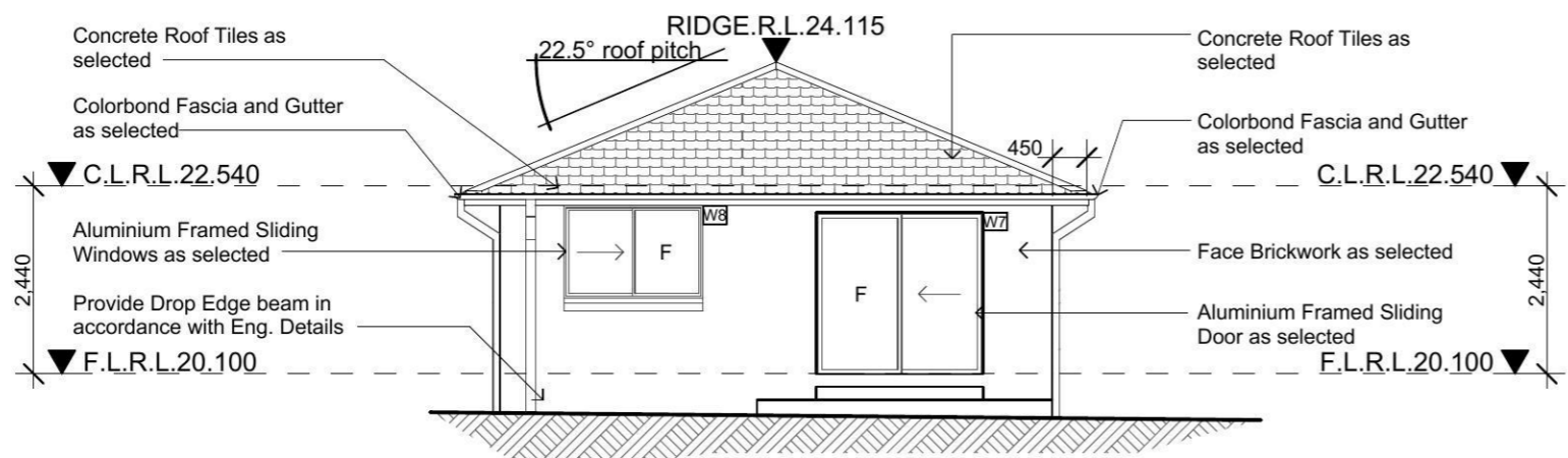
Southern Elevation Dwelling B scale 1:100
