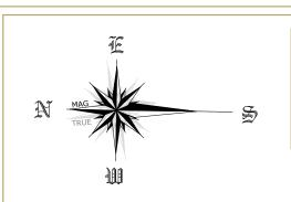
BEARINGS SHOWN HAVE BEEN DETERMINED FROM NSW LAND REGISTRY SERVICES PLANS AND ARE RELATED TO MAGNETIC AND FURTHER INVESTIGATION WOULD BE REQUIRED TO DETERMINE ACCURATE TRUE
