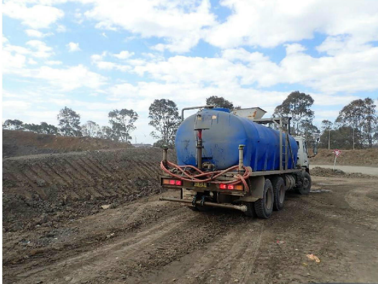
Photograph 10: Volvo 9,000 litre cart with spray bar and water cannon
