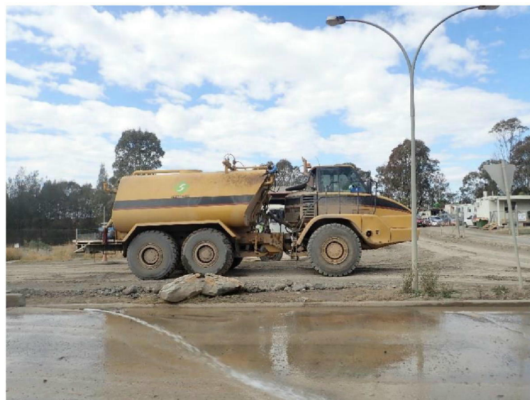
Photograph 08: 30 tonne CAT truck with spray bar and water cannon.
