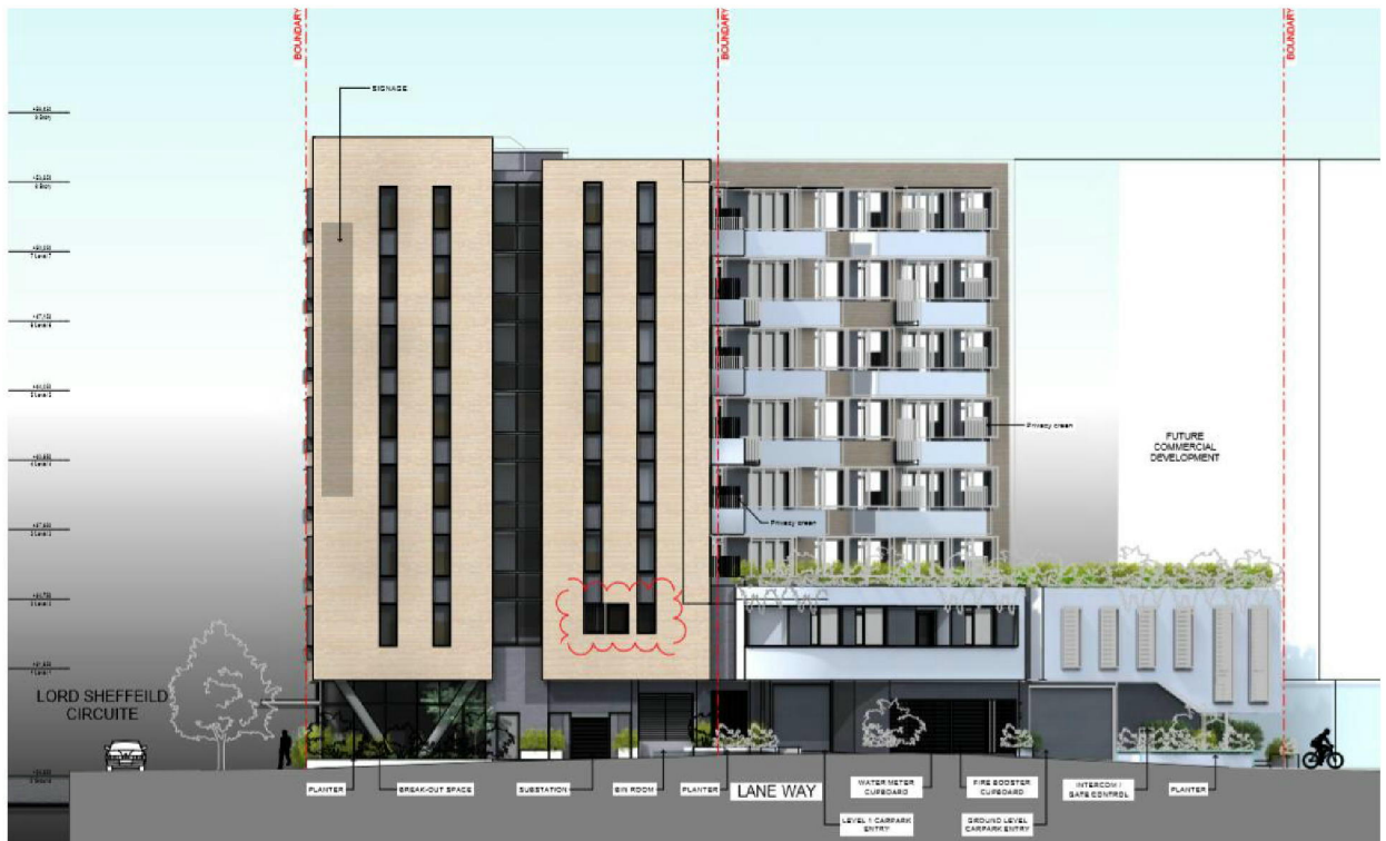
Figure 5 – East Elevation Plan showing the location of the proposed amendment to the window.
