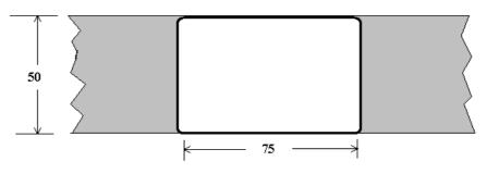
The cleat is made from 50 x 6 flat and has a cut away on each side with a post connecting it to the stringer and the cross rail hook is inserted into it.
