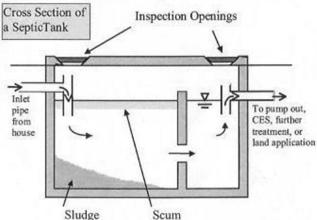
Bacteria in the septic tank break down the solid matter in the sludge and scum layers. Material that cannot be fully broken down gradually builds up in the tank and must be pumped out periodically.
