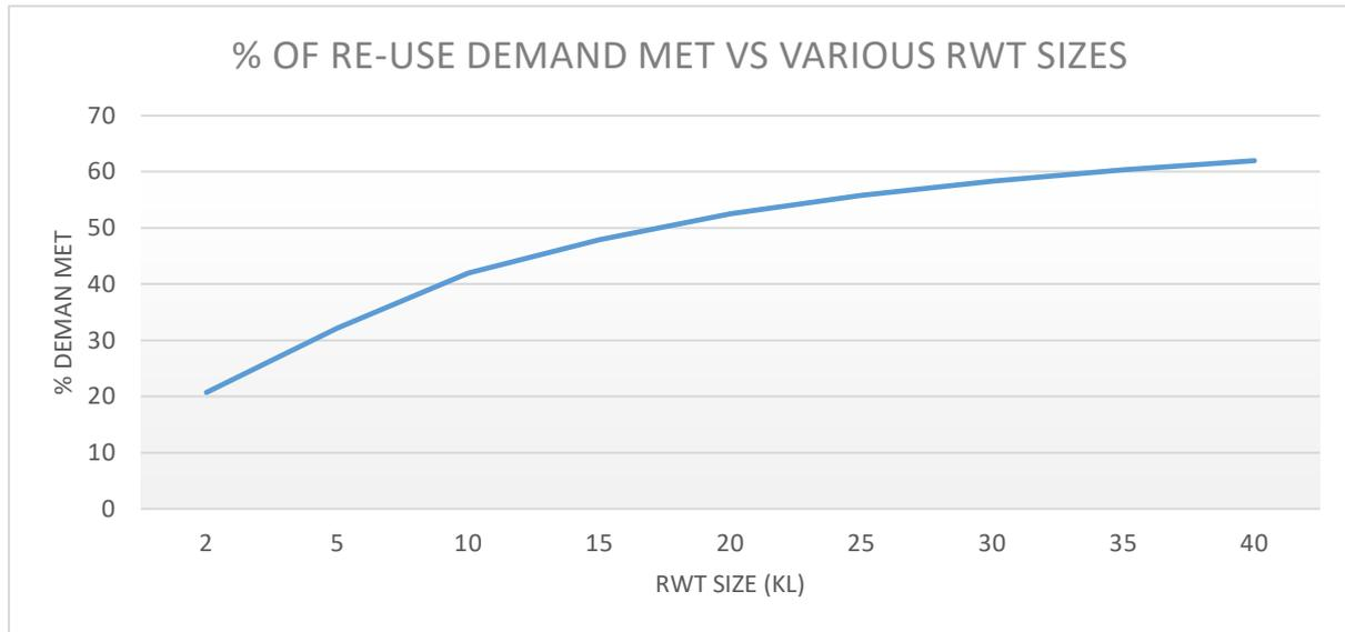
Figure 3: Efficiency Curve based on none potable demand use for 5 toilets and 367m<sup>2</sup> of landscaping area on Ground Floor level
