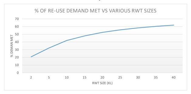
Figure 3: Efficiency Curve based on none potable demand use for 5 toilets and 367m<sup>2</sup> of landscaping area on Ground Floor level
