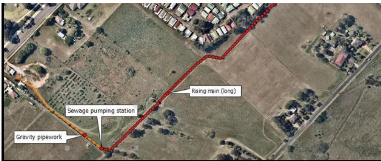
Figure 4 On-Site Package Pumping Station Discharging to the Nepean Shores Development Manhole
