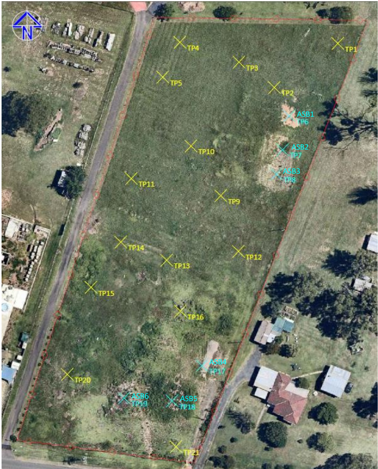
Figure 3: Site sampling plan showing location of the twenty-one (21) test pits (yellow) with the concurrent asbestos sampling (blue). (enhanced image Appendix B).
