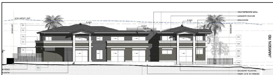
Figure 7: Extract from the development plans showing compliance with the 8.5 metre height of buildings standard.
