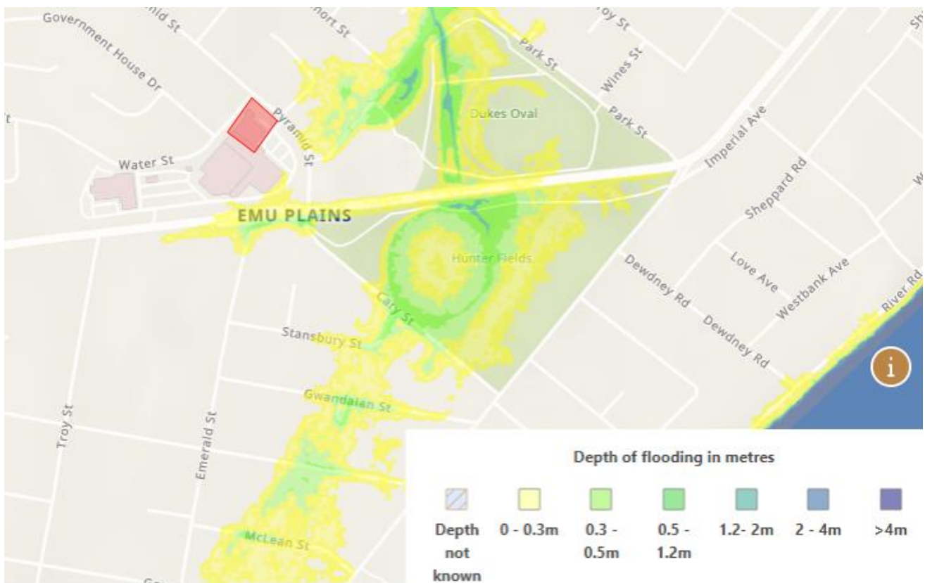
Figure 3 – 100-year flood extent (SES Flood Mapping)
