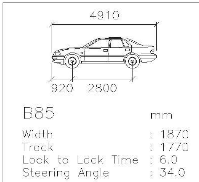
***Figure 11: B85<sup>th</sup> percentile vehicle template (AS 2890.1-2004)***
