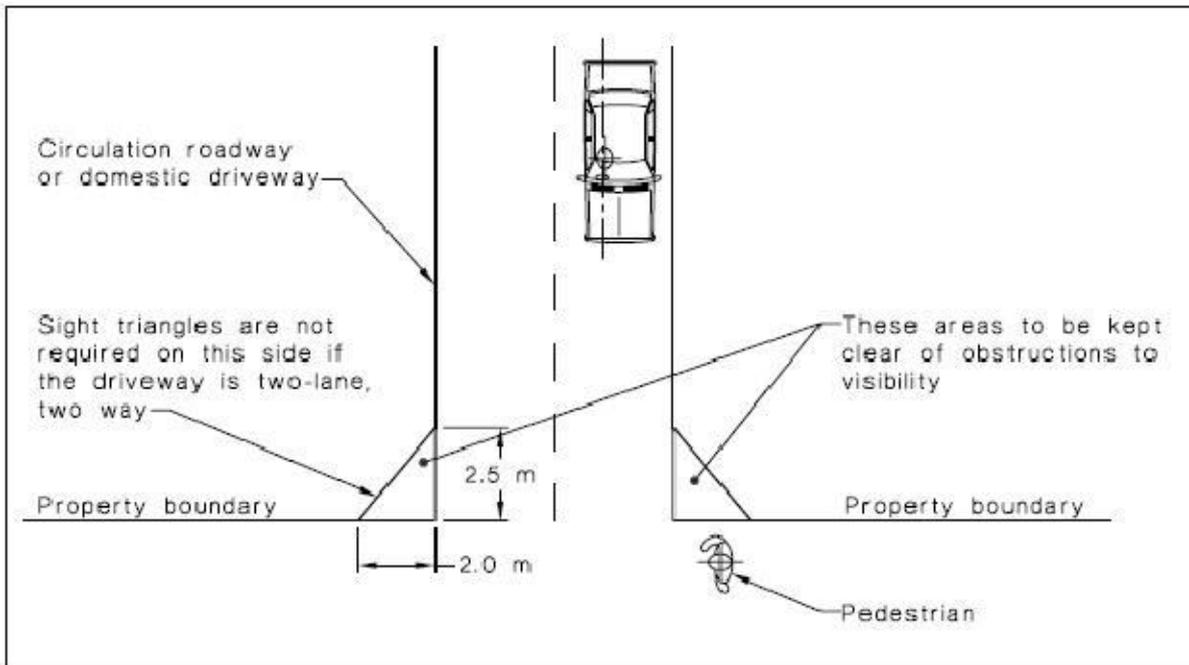
**Figure 9: Minimum Sightlines for Pedestrian Safety (AS 2890.1:2004)**
