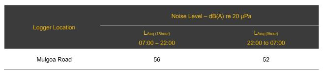
Traffic noise levels recorded by the noise logger have been corrected to account for the distance from the road to the proposed façade. These are representative of the noise levels the proposed façade will encounter.
