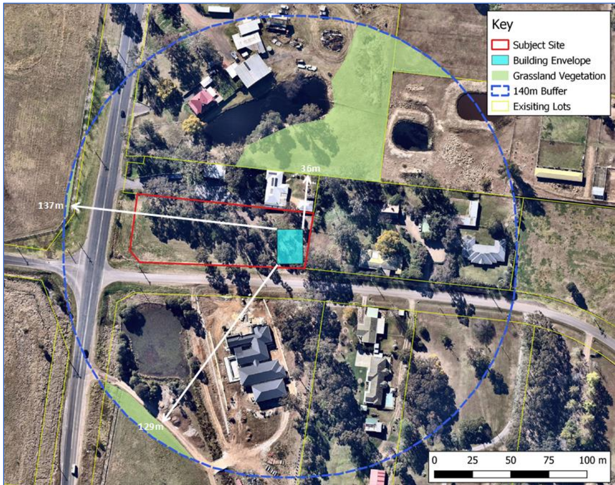
Figure 6. Hazardous vegetation affecting the subject building. Source: NearMap (2021) with overlays by BFCs P/L. Aerial Photography date: x/0x/202x
