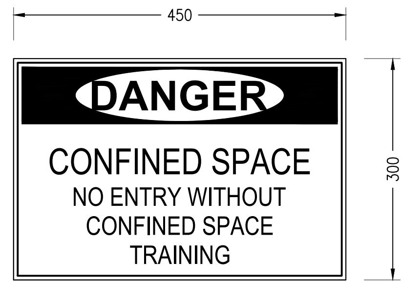
CONFINED SPACE SIGN DETAIL SCALE 1:20
