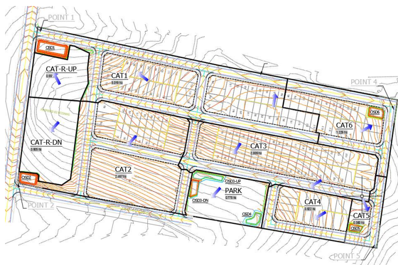
Figure 4- Site catchment areas in post-development condition
