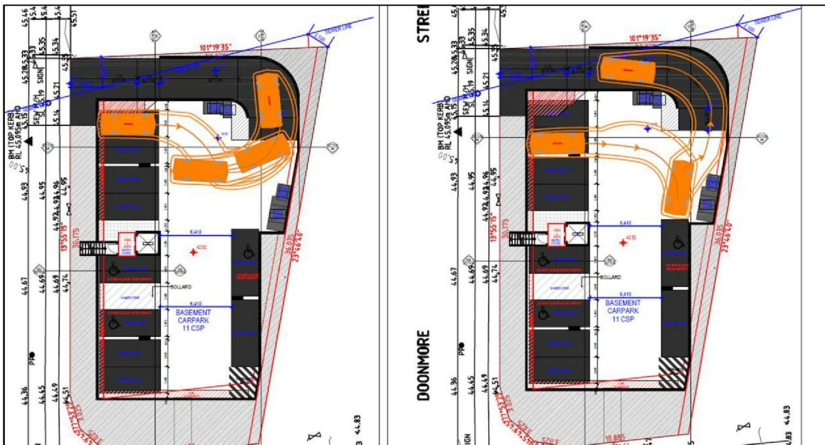
Figure 4-2: Vehicle Swept Path Analysis (Car Parking Space 2)
