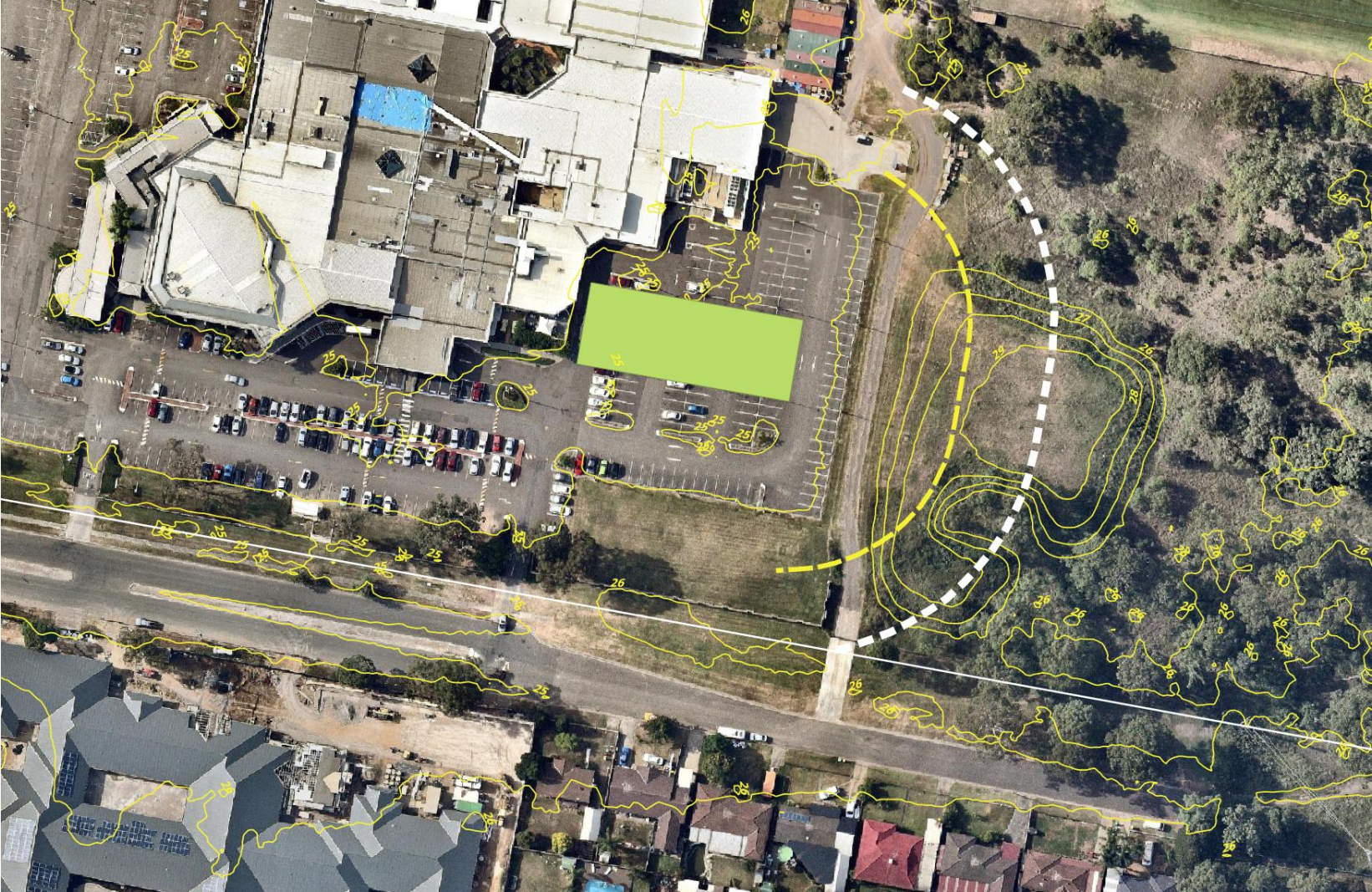
Map 4. The above map shows both a 40m APZ required for Woodland Vegetation and a 60m APZ (white dashed line for forest vegetation). Both can be incorporated into the already managed lands.
