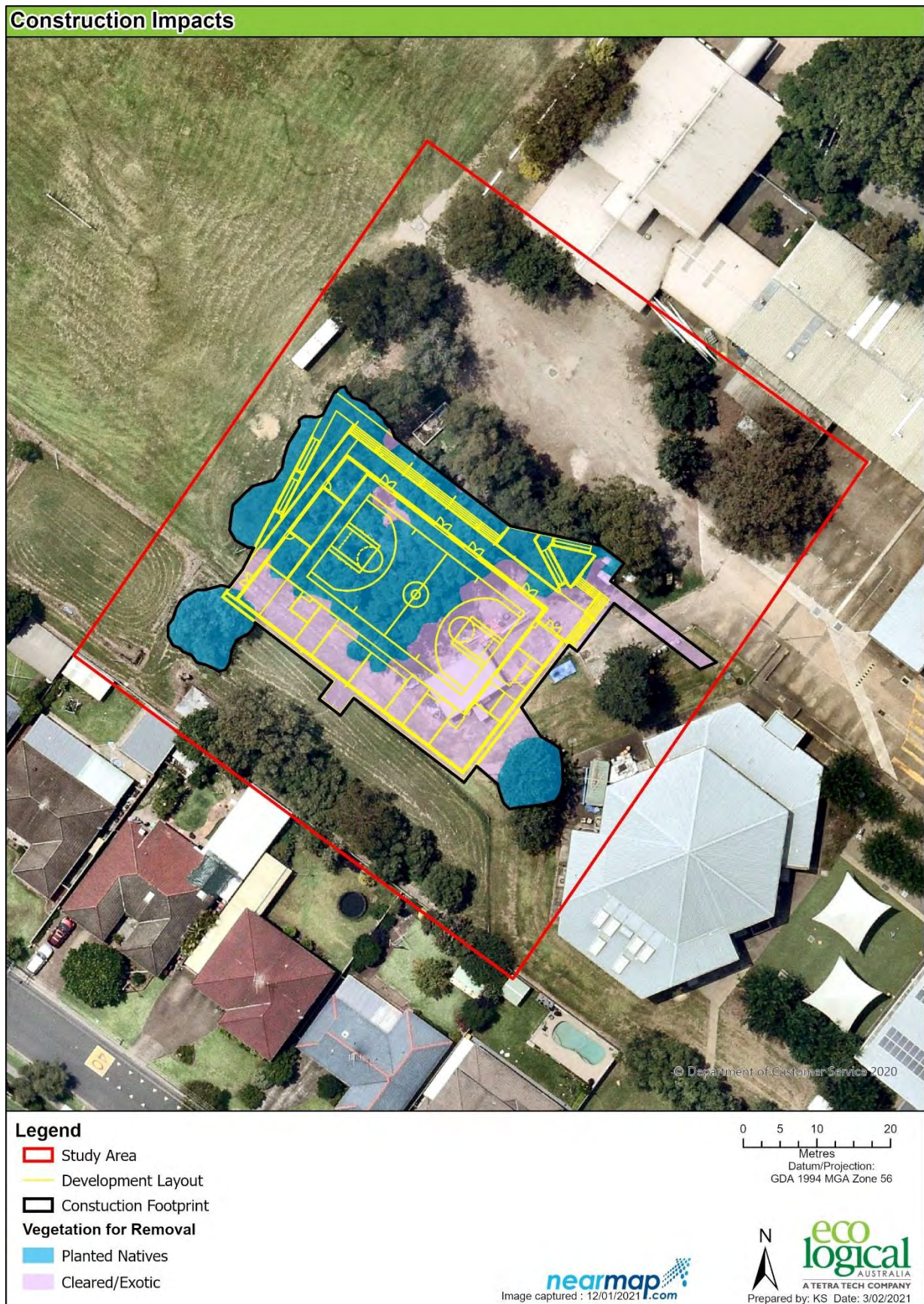
Figure 6: Direct Construction impacts of the proposed works
