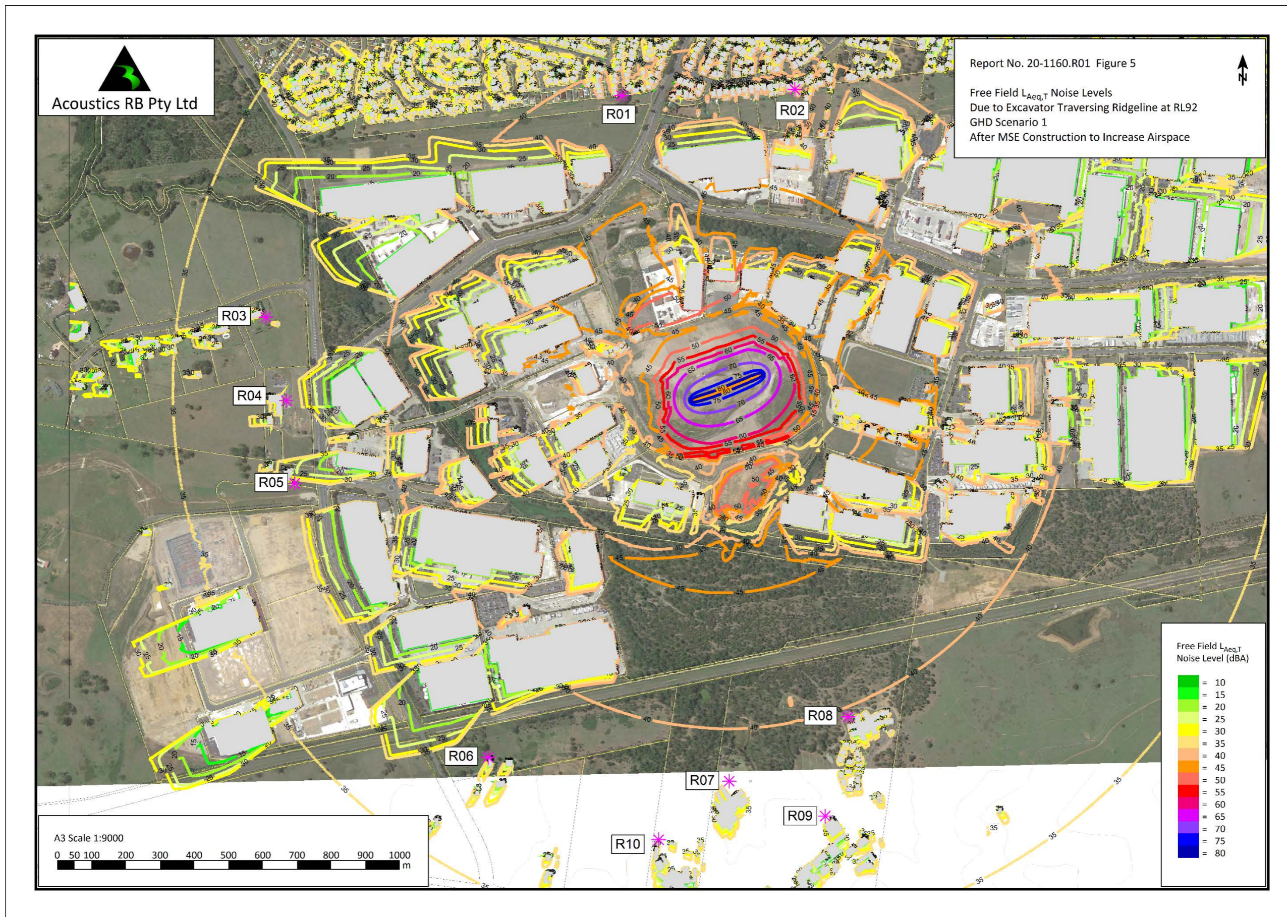
Figure 5 – New Noise Model – Scenario 1 Noise Level Contours After MSE Wall Modification
