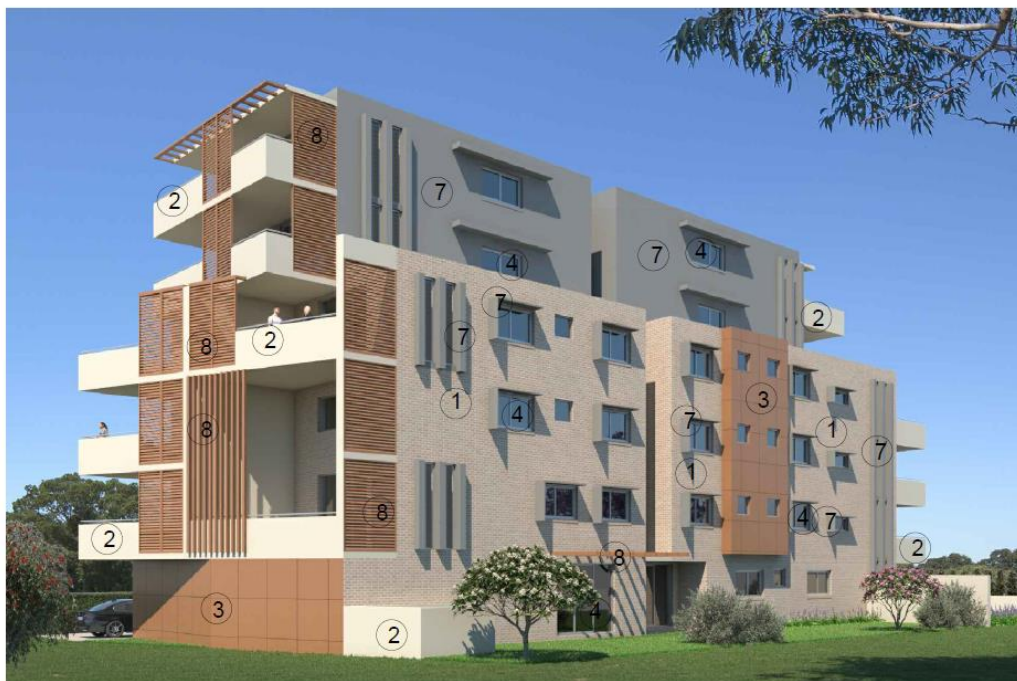
Figure 17 Extract from Architectural Plans – External Finishes (image courtesy of Antoine J. Saouma Architects)
