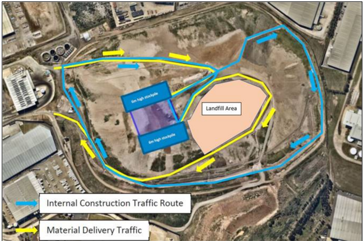
Figure 5: Processing area, stockpile locations and haul routes
