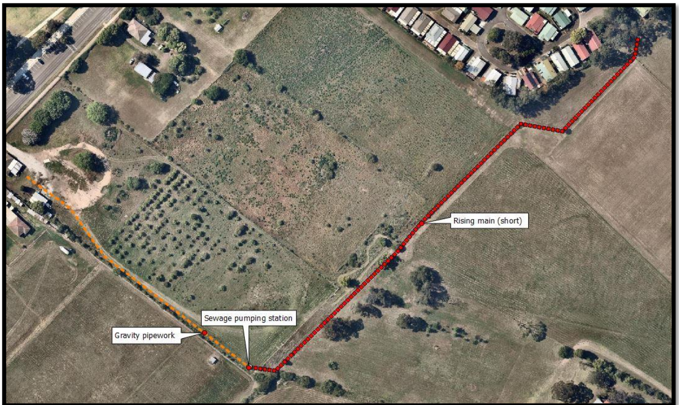
Figure 8 Package pumping station on site discharging to the Nepean Shores development manhole
