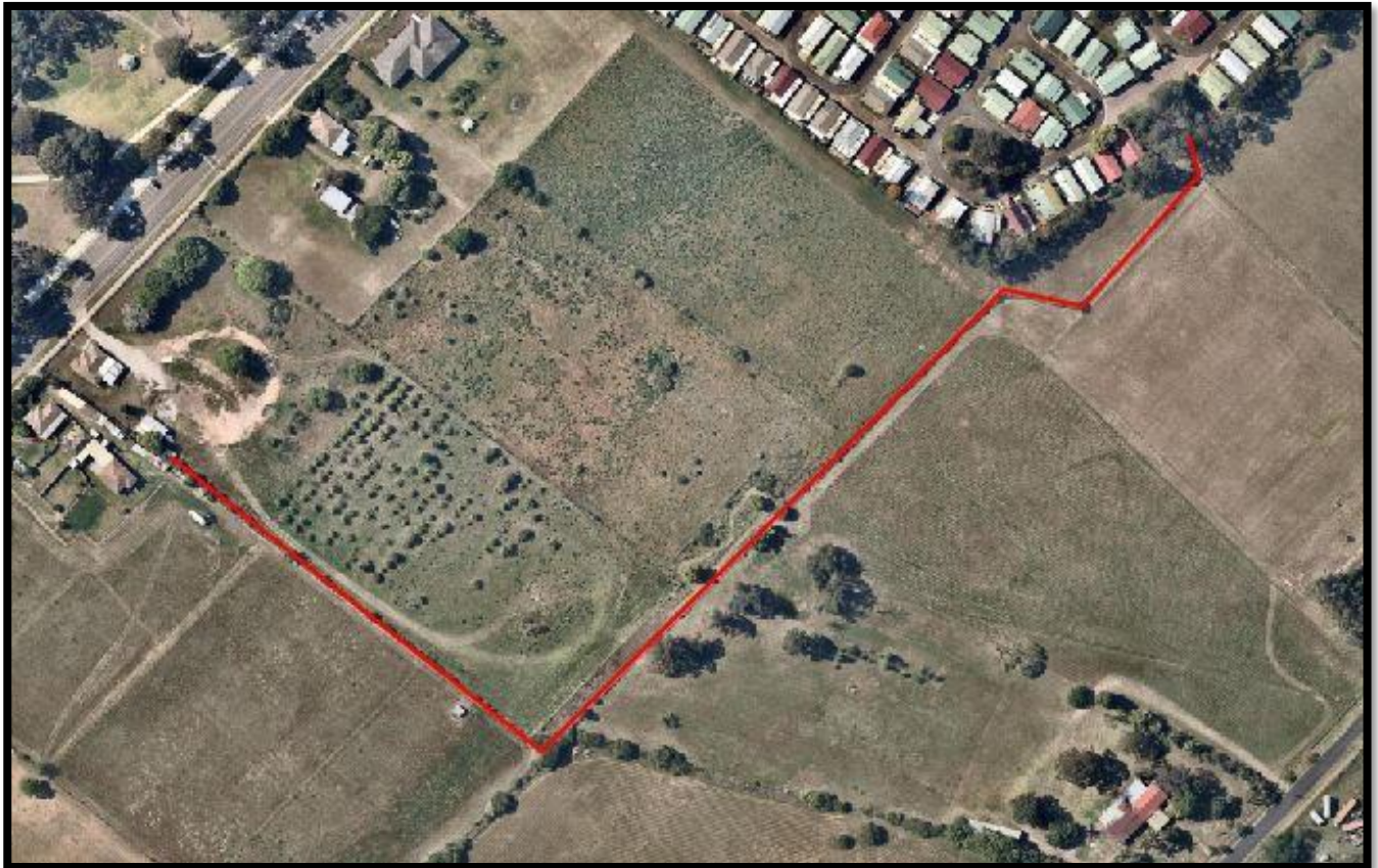
Figure 4 Gravity pipeline route along property boundaries
