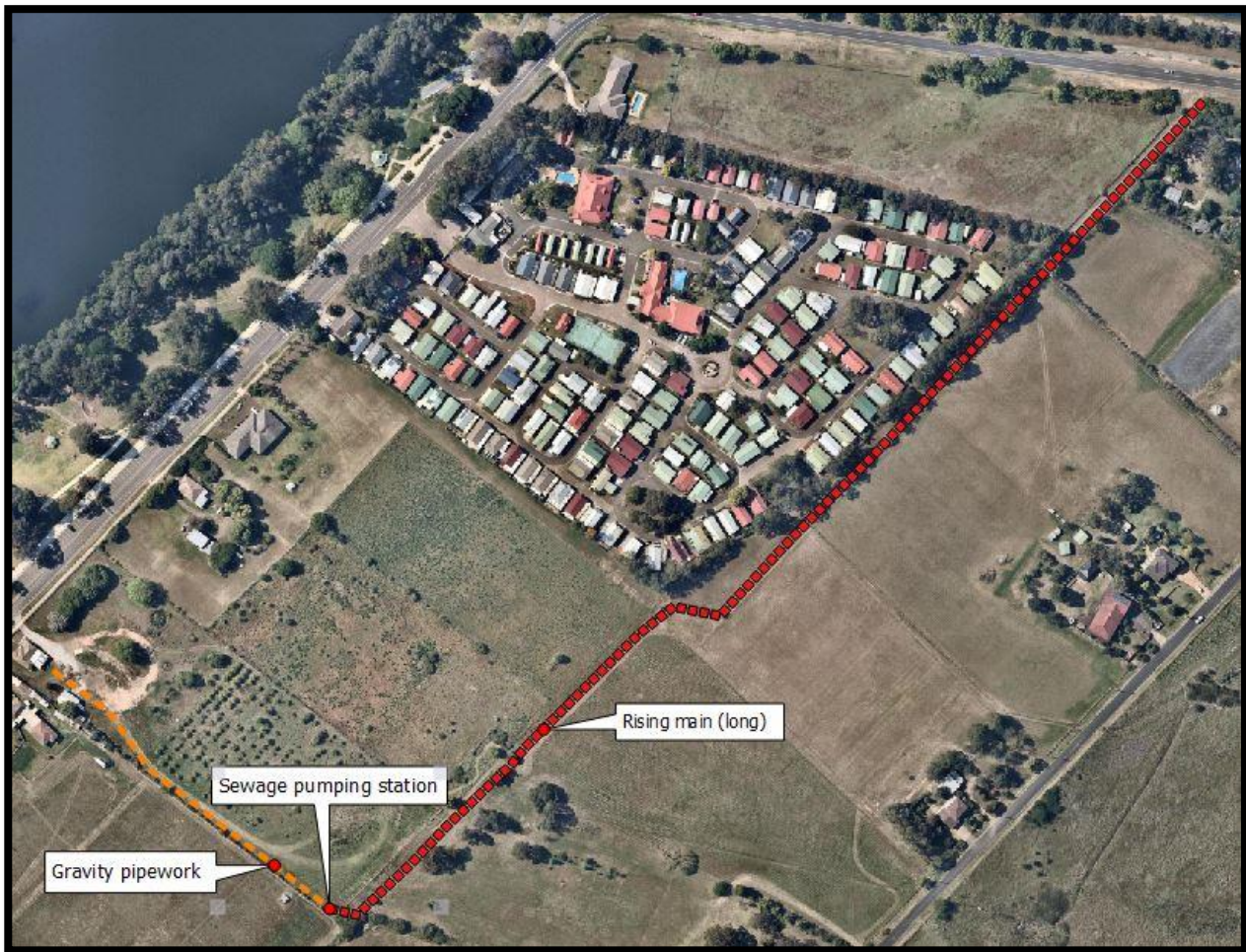
Figure 9 Package pumping station on site discharging to the closest manhole in Jamison Road
