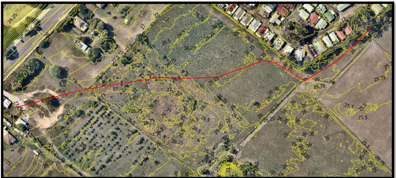
Figure 6 Recommended gravity pipeline route
