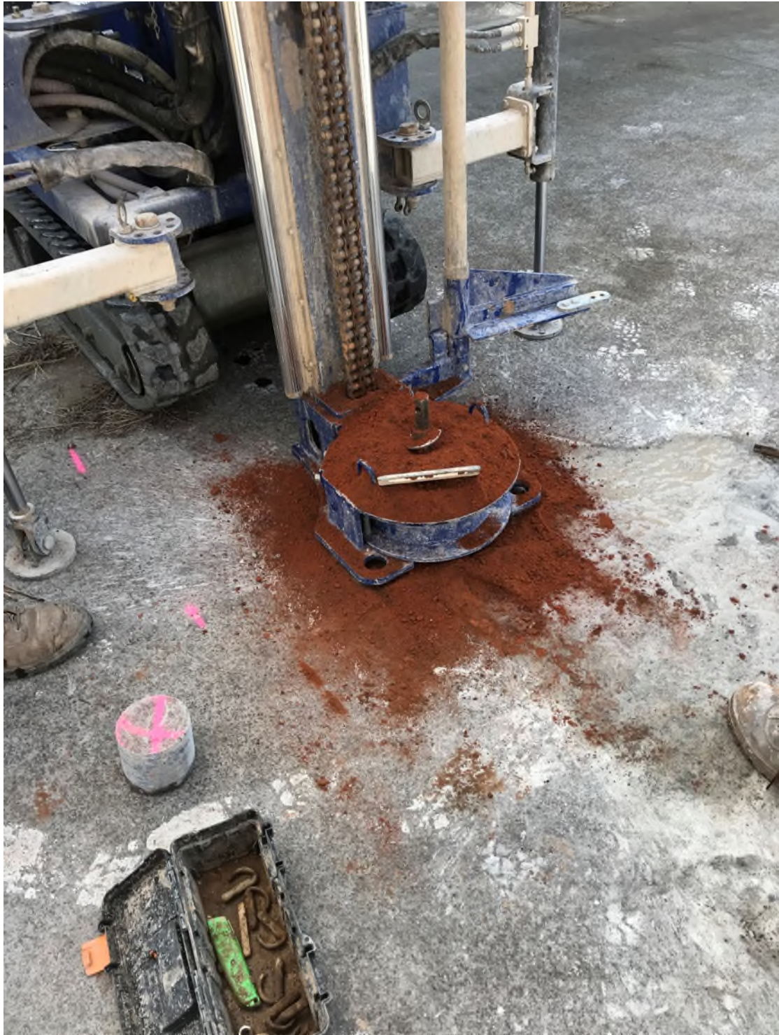
Photograph A3.3: Typical Red Sand beyond gravel fill representative of natural soil profile
