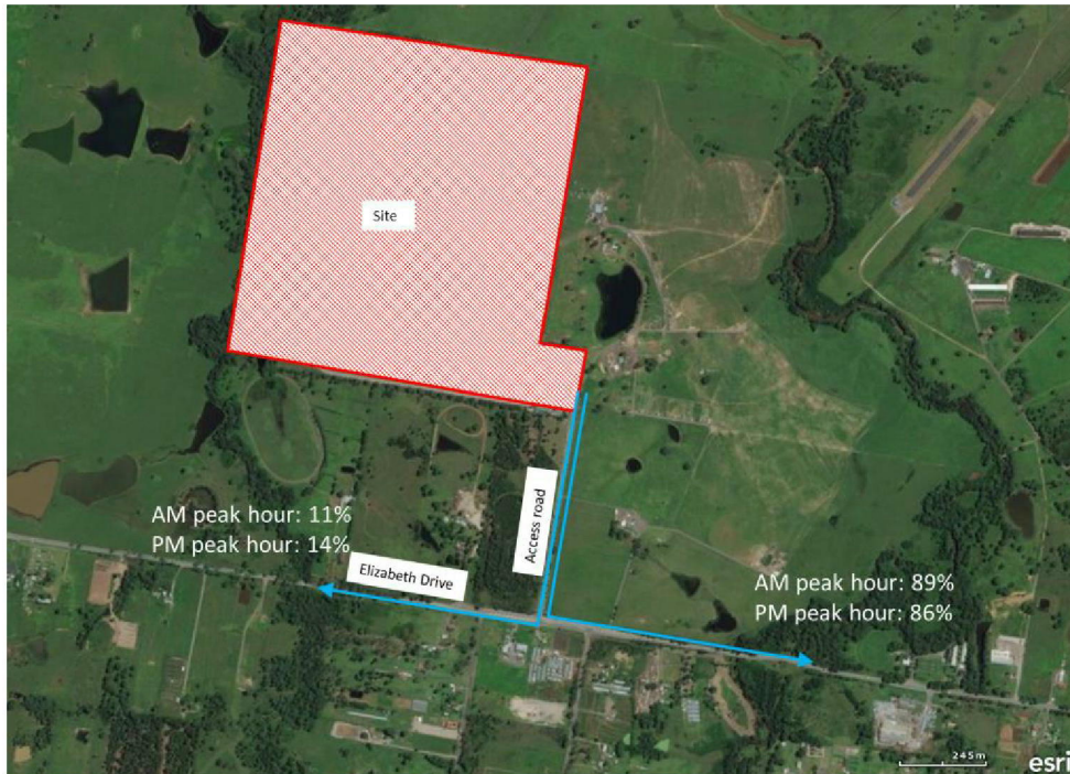
Figure 2.8 – Site egress routes and distribution for heavy vehicles – AM and PM peak hours
