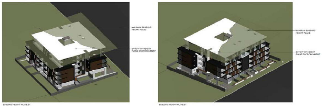
Figure 11 Building height plane - showing the height breach in white
