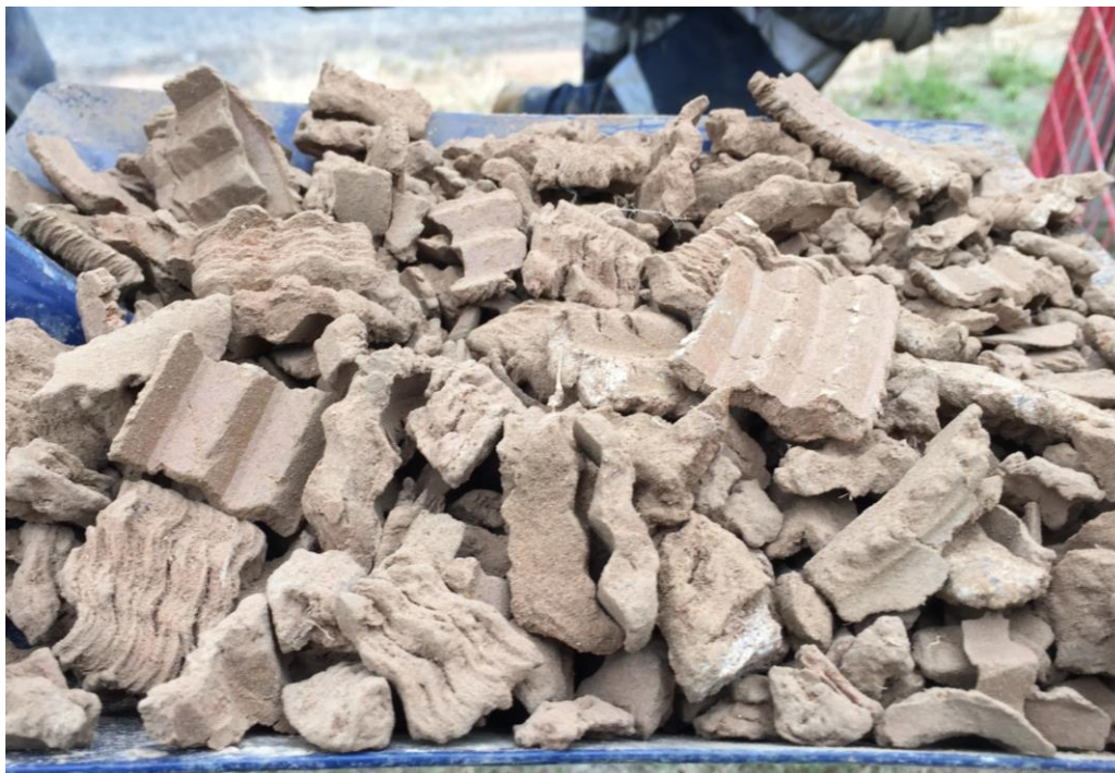
Figure 3 Drill cuttings returned from fill at BH08, approximate depth of 0.5mbgl. Note unusual corrugated shape.
