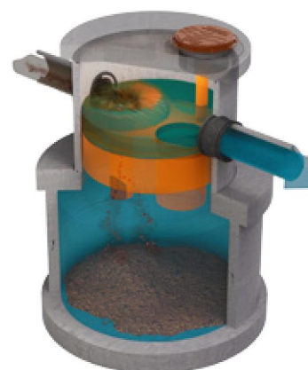
Figure 2 – HumeCeptor® system operation during high flow conditions
