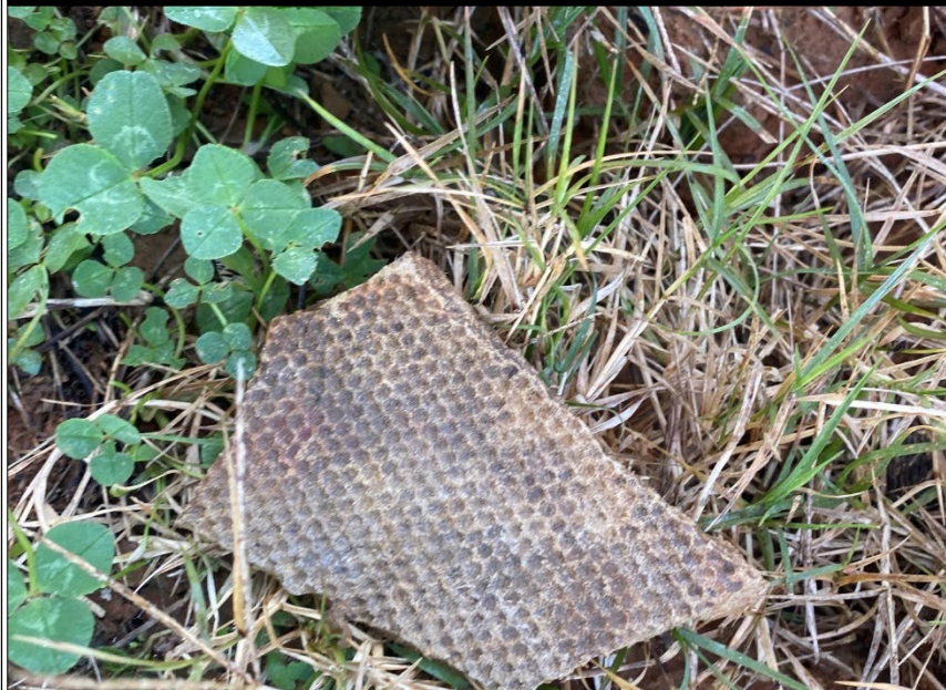
PHOTOGRAPH 16: ACM FRAGMENT TO THE SOUTH EAST OF THE LARGE COMMERCIAL SHED
