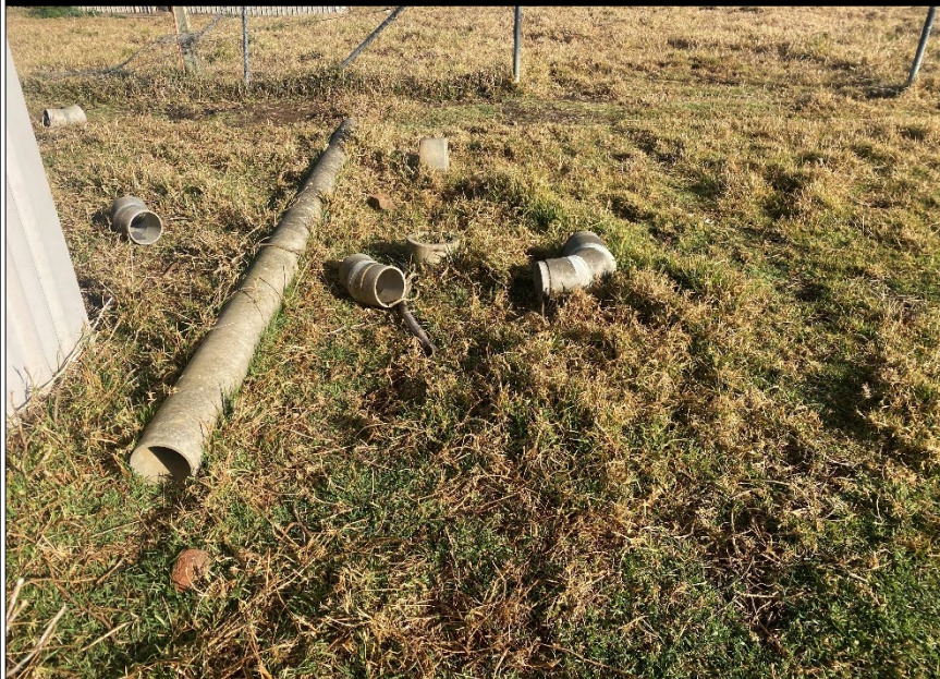
PHOTOGRAPH 15: ACM PIPES ADJACENT SMALLER SHEDS WITHIN CENTRAL PORTION OF SITE
