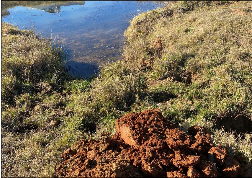
PHOTOGRAPH 20: TP45 ADJACENT SOUTH EASTERN CORNER OF COMMERCIAL SHED. ANTHROPOGENIC WASTE THAT ACM FRAGMENT WAS IDENTIFIED IN AT TOP OF FRAME
