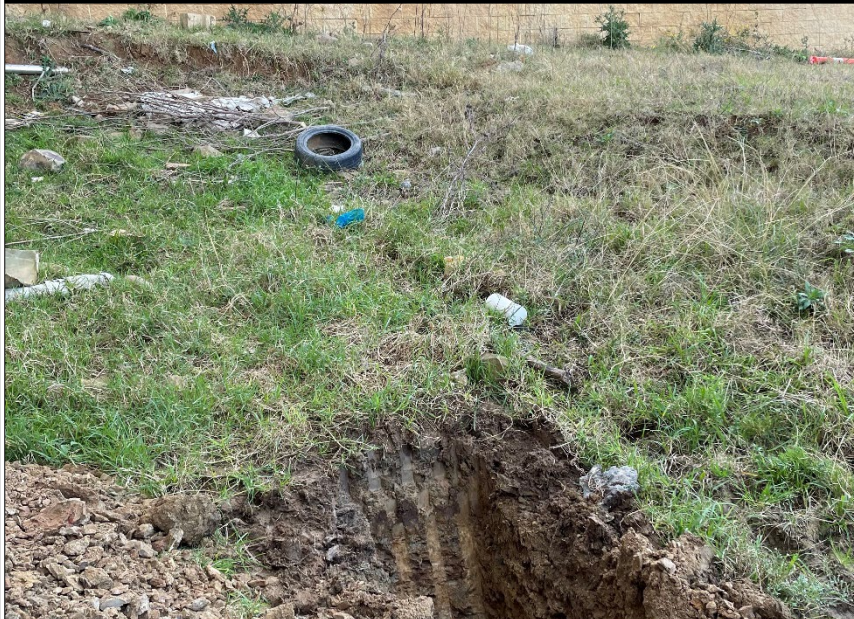
PHOTOGRAPH 20: TP45 ADJACENT SOUTH EASTERN CORNER OF COMMERCIAL SHED. ANTHROPOGENIC WASTE THAT ACM FRAGMENT WAS IDENTIFIED IN AT TOP OF FRAME
