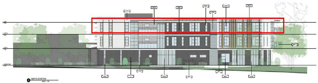
Figure 1: Extract of east elevation indicating the maximum height non-compliance shown in red (Source: MDP Architects)
