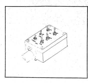
Release "BRAKE" switch. Engage "HYDRAULIC PUMP" switch and make sure motor is running in the correct direction (indicated by an arrow on the pump).
